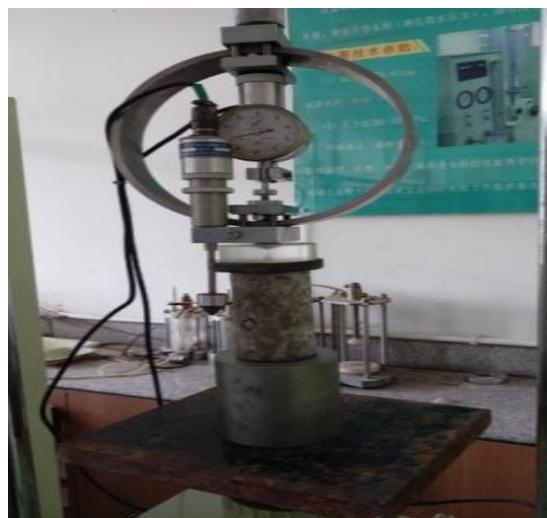
Fig.3 Unconfined compressive strength testing machine
